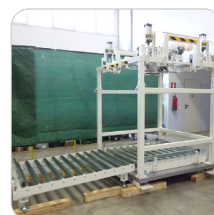
Big bags filling station
