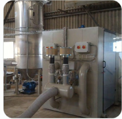
Vacuum pump unit & receiving cyclone / filter (continuous)
