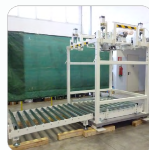
Big bags filling station
